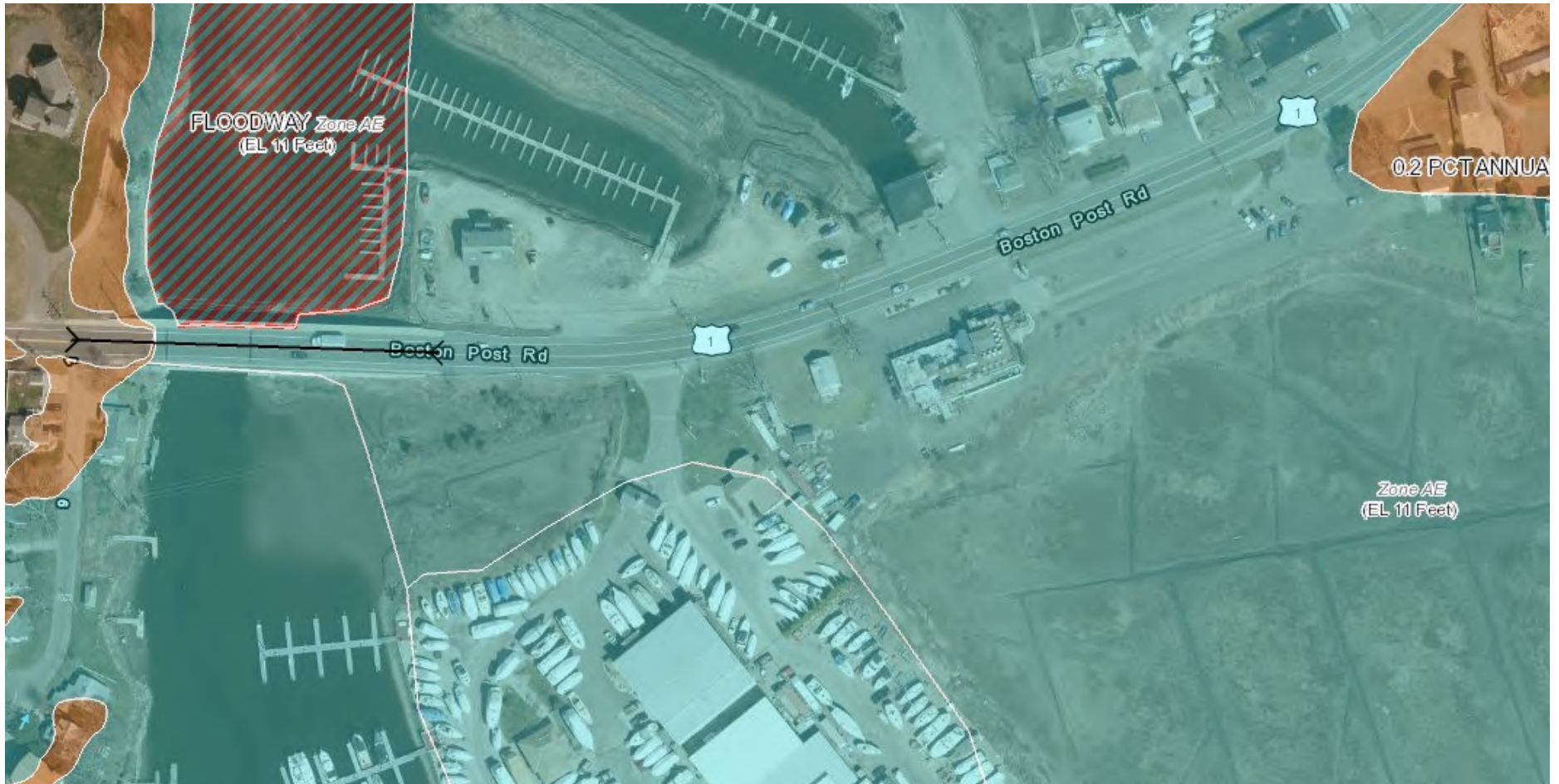
Figure 3-10: FEMA Special Flood Hazard Areas (SFHAs) at Route 1 Bridge over the Menunketesuck River.
